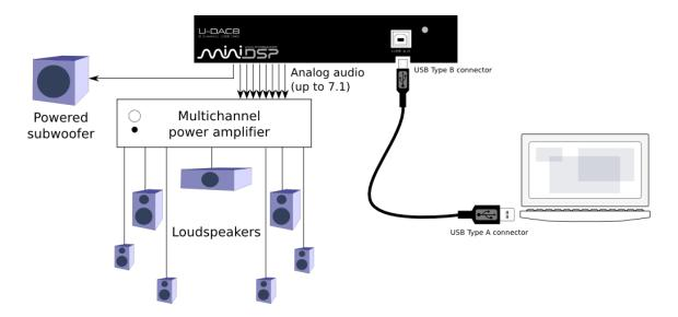
The outputs of the U-DAC8 can also be connected to any device with multichannel analog inputs, such as an A/V receiver or processor:
