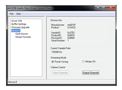
The current sample rate shown reflects the sample rate of the file being played by the Windows player. This setting cannot be changed in the Control panel, but simply reflects the current sample rate of the U-DAC8.
